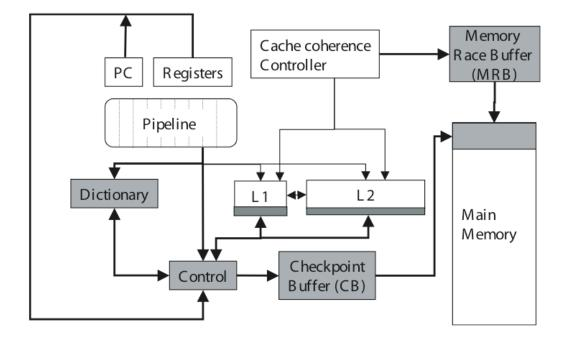
Figure 2.1: BugNet's architecture [SNC05]
