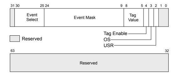
Figure 6.1: Layout of the ESCR register [1005]
